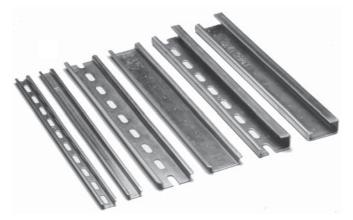
Kinematics offers full lengths of three standard D.I.N. rail cross-sections, in both perforated and non-perforated styles. Kinematics' Smart-Blocs® will mount directly to any of the three styles. Rail material is zinc-plated steel with a yellow chromate finish. Standard rail length is 2 meters (6'-6").
