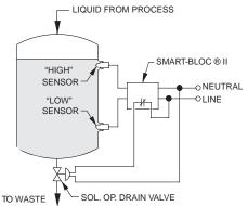
are "DRY". Refer to the adjacent schematic. On start-up, the tank is empty and both sensors are "DRY". No action occurs because the relay contacts are open. As the process fills the tank, the liquid level eventually rises to a point
