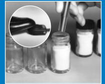
**INSERT THE GUN** into the mouth of the container to be filled. Depress the foot switch. Vacuum changes to gentle pressure, discharging another perfect, dust-free dose.
