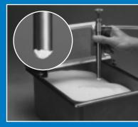
DIP THE GUN into the product trough. Powder is instantly picked up into the barrel at a controlled, even density.
